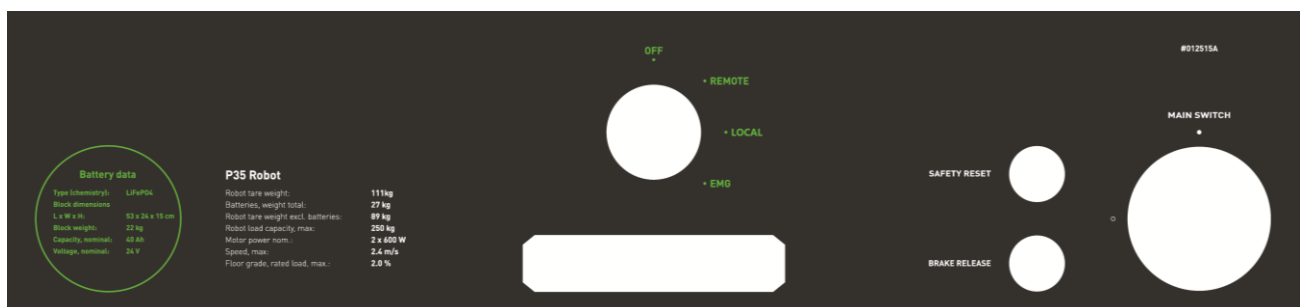
Figure 12 P35 foil sticker at rear side
